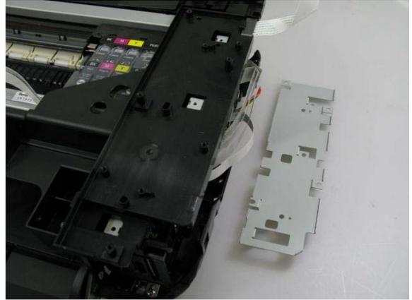
7) Remove the main case and sub-case (1 screw).
