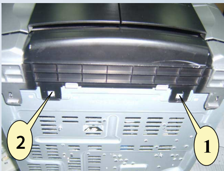
7.Pull the hook at 1 and 2 of and separate ASSY-FRONT
