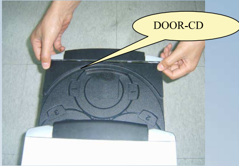
1. Power on and open the disk, Separate Door-CD
