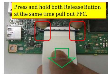
FFC connector broken if pull out FFC without press and hold both Release Button of connector. Symptom 5X blinking will be appear due to improperly seated.
