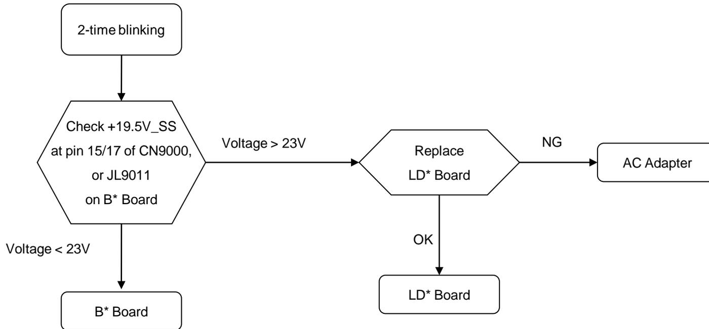
3-2-1. LED Blinking: 2x (Main power Error)
