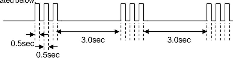
Example: The figure above shows LED display when SHUTDOWN is caused by Audio Error. It repeats flashing for a specified number of times in 0.5sec/cycle and has a 3 seconds interval of lighting off. Please note that a 3 seconds interval of lighting off is fixed regardless of abnormal state types.
