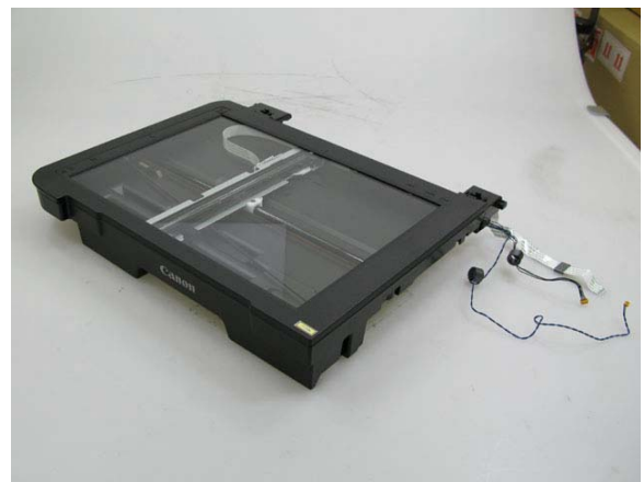
Disconnect the FFC and the harness, and remove the core (red-circled).
