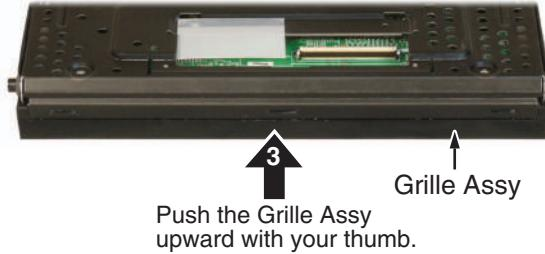
**4** Release the three latches on the upper side of the Grille Assy with your left hand.
