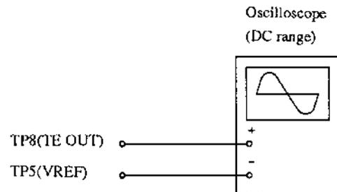
1. Connect an oscilloscope to test points TP8 (TE OUT) and TP5 (VREF).
