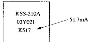
$$\text{Laser current } I_{op} = \frac{\text{Voltage across R4}}{10\Omega}$$
