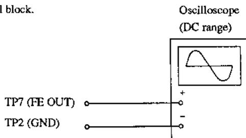
1. Connect an oscilloscope to test points TP7 (FE OUT) and TP2 (GND).
