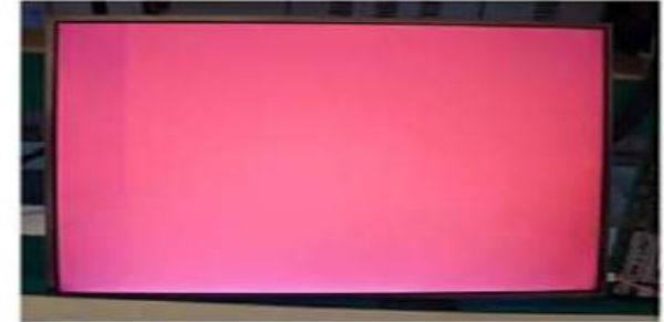
Vertical Block Source TAB IC Defect
