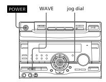
→ Press and hold WAVE to start the Wave function, and release to resume normal listening.
