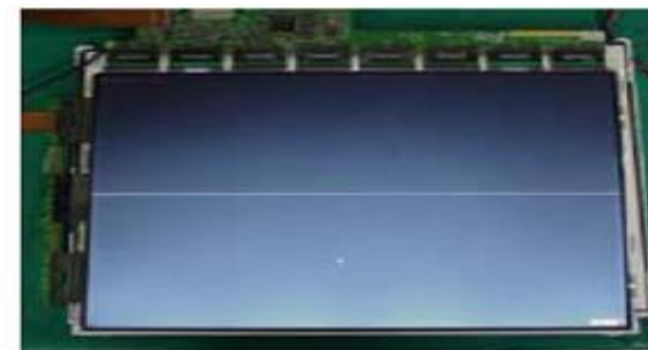
Horizontal line Gate TAB IC Defect
