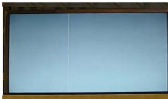
Vertical Line Source TAB IC Defect
