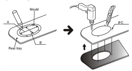
If it will be necessary to cut steel, reinstall the cosmetic panel in place and use the hole you have previously cut as a template. This will help to insure proper cutting and a good fit. Now, mark the locations for the speakers mounting screws, remove the panel and drill the screw holes. When finished you may replace the panel.
