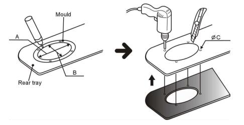
If it will be necessary to cut steel, reinstall the cosmetic panel in place and use the hole you have previously cut as a template. This will help to insure proper cutting and a good fit. Now, mark the locations for the speakers mounting screws, remove the panel and drill the screw holes. When finished you may replace the panel.
