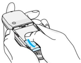
Locate the SIM card socket in the back of the phone. Follow the steps below to install the SIM card.
