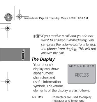
numbers. **⋈**•) Signal Strength. The more segments displayed in the bar graph, the better the signal strength.
