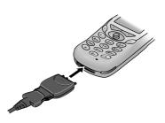
3 Plug the other end of the cable into the serial interface connection on the external device and tighten the screws.
