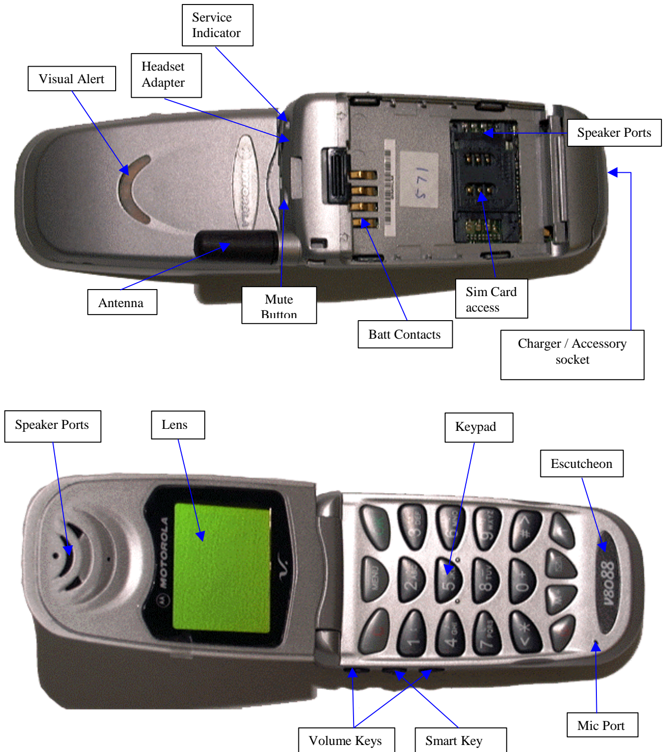
Fig 2.1 Mechanical pictorial Overview
