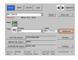
[13] Configure the advanced settings depending on the input signal and press the "Exit" button.
