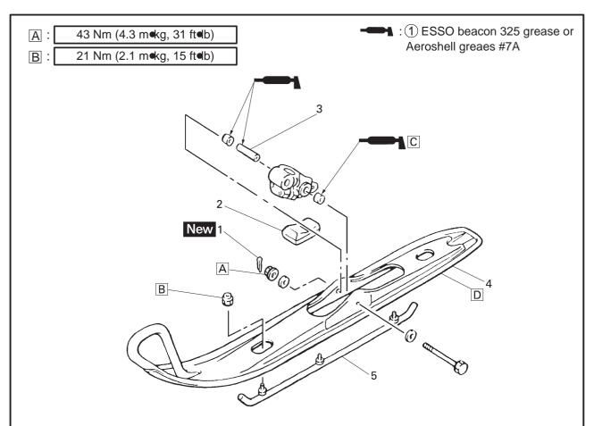
$\overline{\mathbb{C}}$ : Fit the stopper with its raised portion positioned in front.
