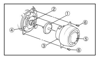
•Fit the end of the adjusting ratchet ① into the adjusting screw ②, and align the cut in the guide ③ with the projection of the stationary cover ④, then install the guide ③, which is fitted to the end cover ⑤ twisting the end cover clockwise approximately 30 degress and tighten the screws (end cover) ⑥.
