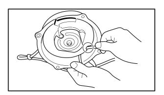
8. Pull about four inches of starter rope from out of the cutout portion in the sheave drum, and rotate the sheave drum five times counterclockwise to preload the starter spring.
