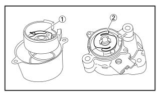
•Lubricate the one way locks 1 ① and 2 ② with a lithium grease.
