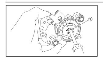
•Screw in the adjusting screw ①, and when it contacts lightly with the end of the back up plate, then back out the adjusting screw ① 1/2 to turn.
