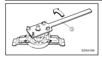
•Tighten the spider to specification using the clutch spider separator (bar wrench) ③.
