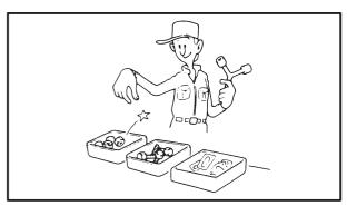
6. Be sure to keep to the tightening torque specifications. When tightening bolts, nuts, and screws, start with those that have larger diameters, and proceed from the inside to the outside in a crisscross pattern.
