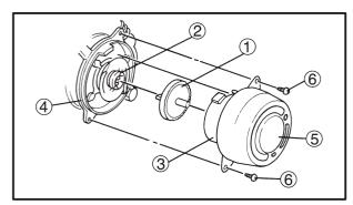
•Fit the end of the adjusting ratchet ① into the adjusting screw ②, and align the cut in the guide ③ with the projection of the stationary cover ④, then install the guide ③, which is fitted to the end cover ⑤ twisting the end cover clockwise approximately 30 degrees and tighten the screws (end cover) ⑥.
