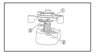
•Align the projection mark ① on the lever with the "86" mark ② on the caliper body, screw the lever ③ counterclockwise to the caliper body.
