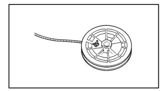
2. Pass the starter rope end into the sheave drum, and knot the rope end. Then fit the knot into the cutout in the sheave drum.
