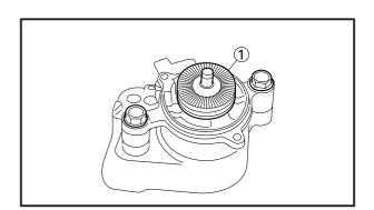
•Removing the adjusting ratchet ①.
