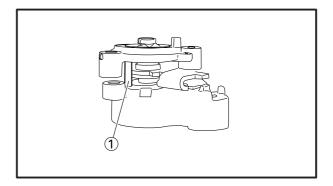
•Install the stopper pin ① into the holes on the caliper body and stationary cover, then tighten the bolts (stationary cover).
