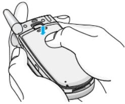
2. Then push to the half of the battery into position.
