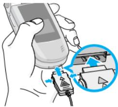
1. With the arrow facing you as shown in the diagram push the plug on the battery adapter into the socket on the bottom of the phone until it clicks into place.
