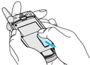
Locate the SIM card socket in the back of the phone. Follow the steps below to install the SIM card.
